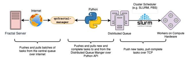
The different levels of communication are all established automatically once the user configures the manager, and this image shows how information flow from point-to-point.
