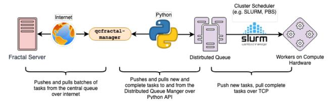
The different levels of communication are all established automatically once the user configures the manager, and this image shows how information flow from point-to-point.
